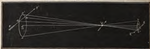
Fig. 37.—Illustrating the connection between the passage of Venus over the sun's face, and the passage of the earth through Venus's shadow-cone.
