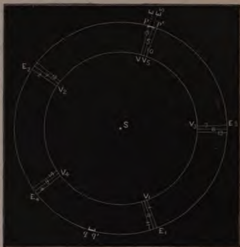
Fig. 18.—Illustrating the regression of the conjunction-lines over a transit region ( pp' ).
